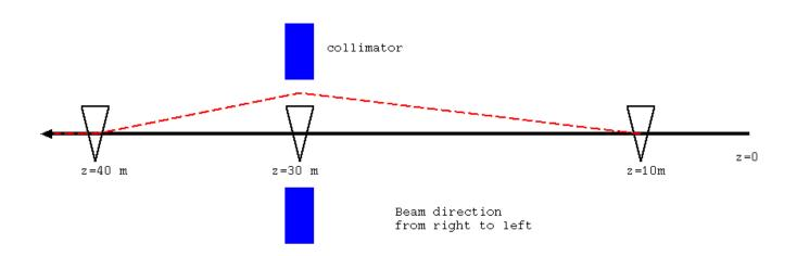
2. Thirty meter downstream of the starting there is a collimator. Assume that the collimator is infittely short in these exercises. What is the beam size at the collimator assuming the initial beam from part 1? There are no magnetic beam optical elements between z=0 and 30 m.
