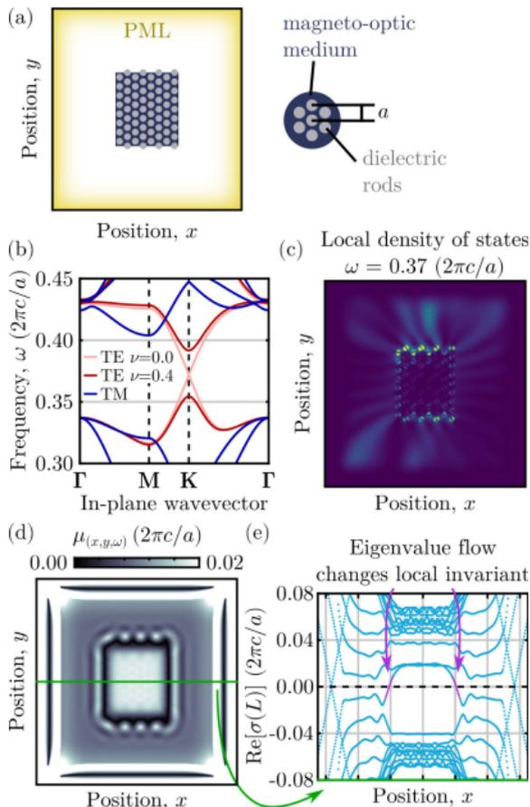
(a) A photonic crystal with Perfectly Matched Layer to simulate light lost to free space.
