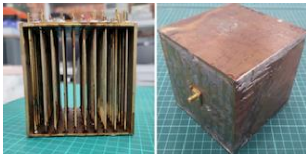
Prototype 10x10 array (11.4 GHz)
