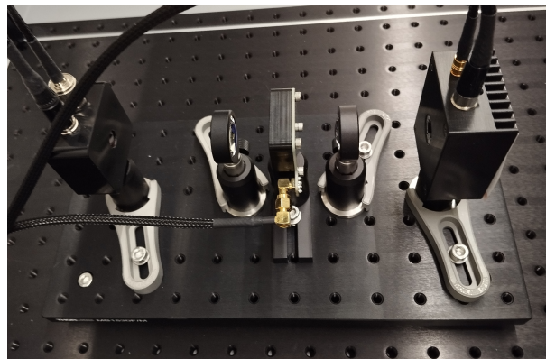
Figure 4: Optical table setup for NV center magnetometry with labels.
